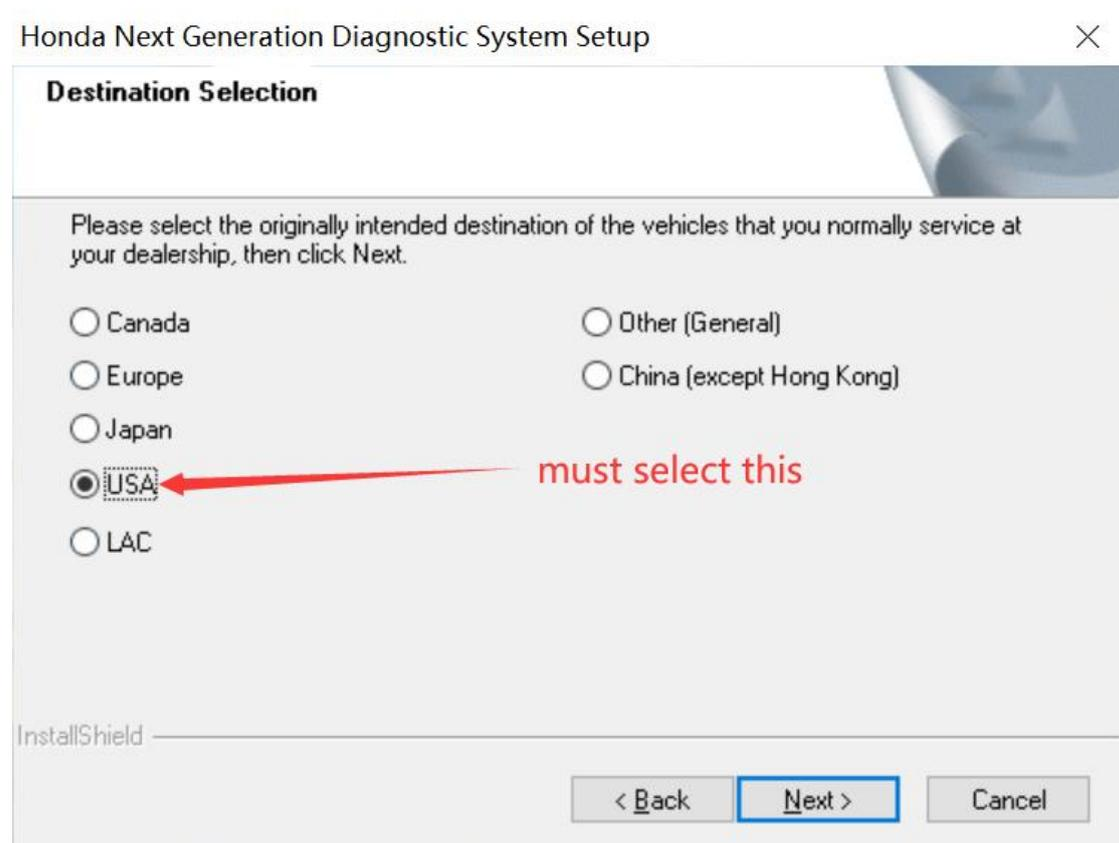
4. After the installation is complete, the first time you run the HDS software, you need to change the interface settings to use the VNCI NANO device.
